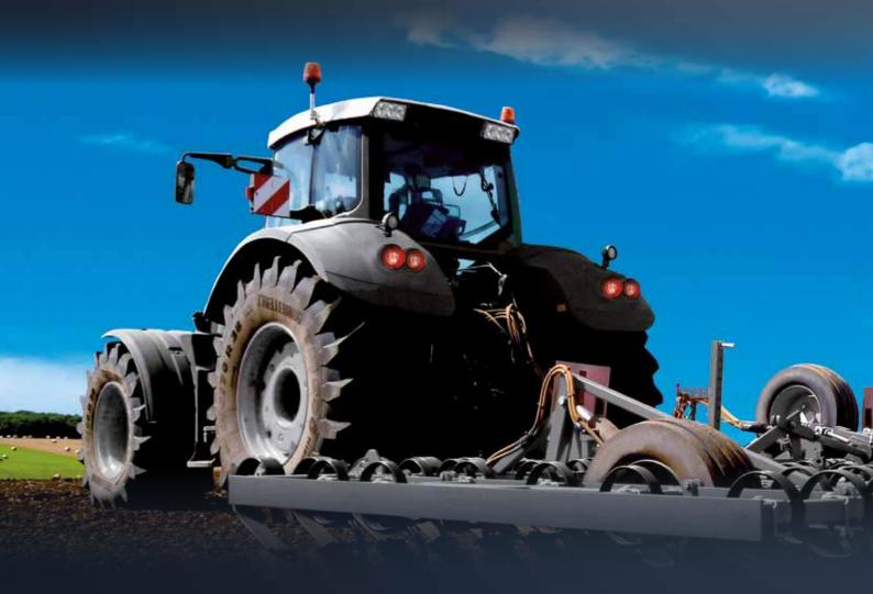
Co-designed with the main agricultural machine manufacturers, the TM900 High Power equips FWD tractors from 250 to 400 hp at speeds of up to 65 km/h $^{*}$ . It offers great traction, excellent self-cleaning capability, premium comfort and handling, minimum soil compaction and low fuel consumption.
