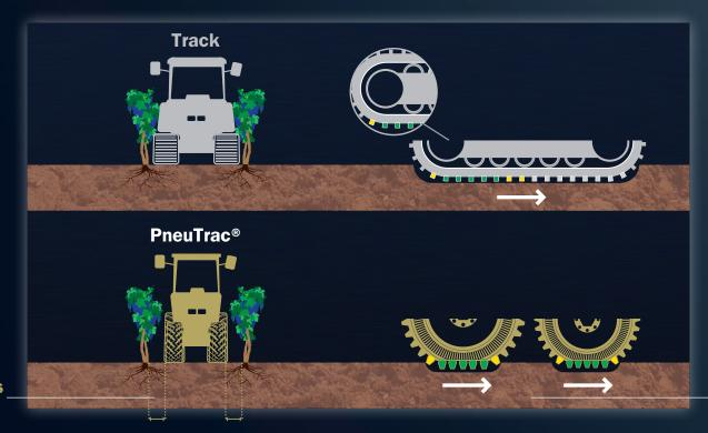
Reduced tractor width and 20% lighter for roots protection vs. track
